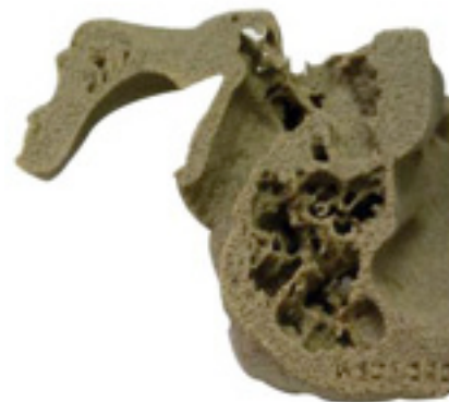
Mastoid form created through the OXPEKK® OsteoFab™ manufacturing process
