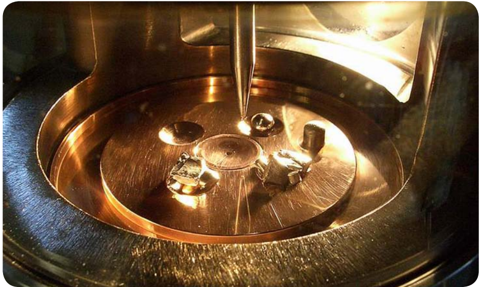
Arc melter in which a plasma of up to 3000°C is produced between a tungsten tip (center) and a water-cooled copper plate/ETH Zurich
