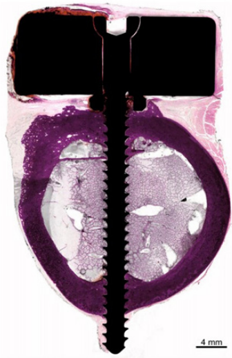
Cross sectional histology image of an antibacterial coated Onkos surrogate implant and screw demonstrating bone and soft tissue apposition in an ovine femur. / Source: Onkos Surgical
